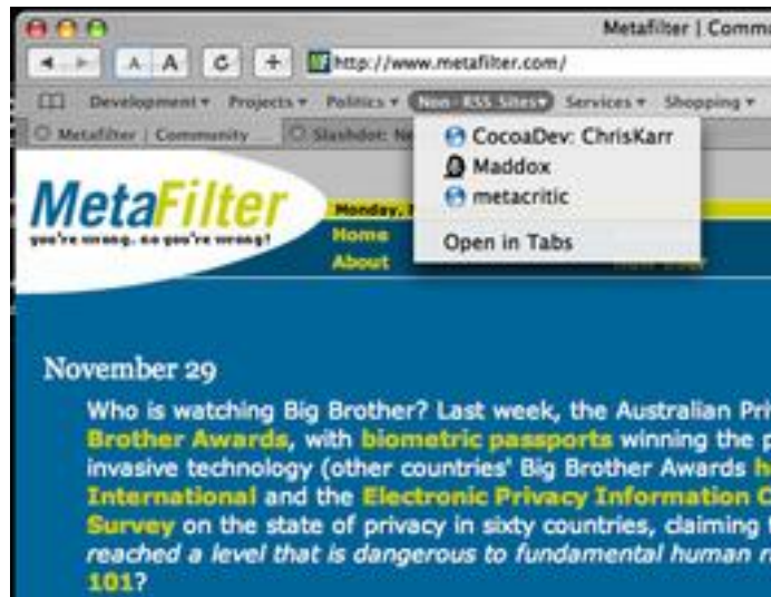
Fig. 1: Safari (Apple) is a Cocoa browser using the brushed-metal theme. It uses standard Cocoa widgets and styles, but does not make use of customizable toolbars or other advanced Cocoa UI elements
